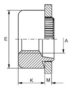
Female thread A = M3,5Height K = 3.0Outer diameter E = 7.0
